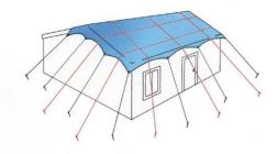
• Nailing of screwing strips to a metal roof will permanently damage the roofing surface. It is only recommended where the metal roof is missing or where it is severely damaged.
